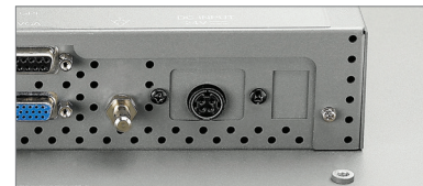
Optional DC input or built-in low-voltage medical grade power supply allows for installation flexibility
